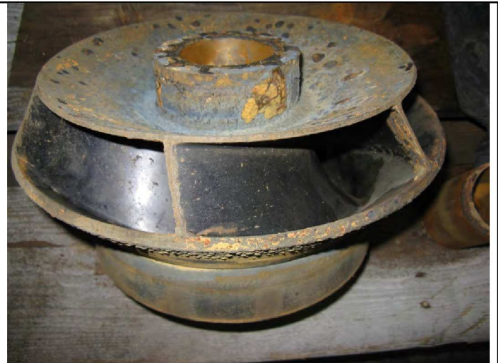
Picture #15 Side view of Impeller. A dynamic-balance to be done upon reuse.
