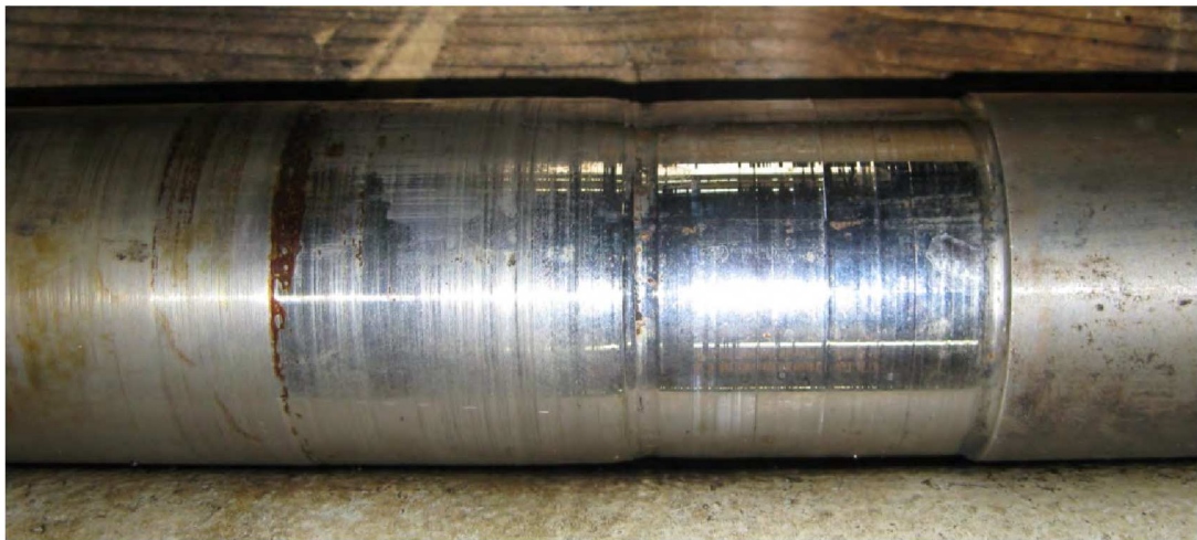
Picture #17 Bowl shaft bearing indicates wear and will need to be replaced. Measure values in Appendix A.
