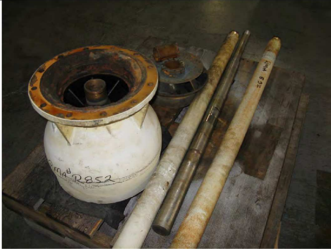
Picture #12 Bowl and oil tube disassembled. Reuse with bowl bearing replacement. Recommend external blast and coat on bowl
