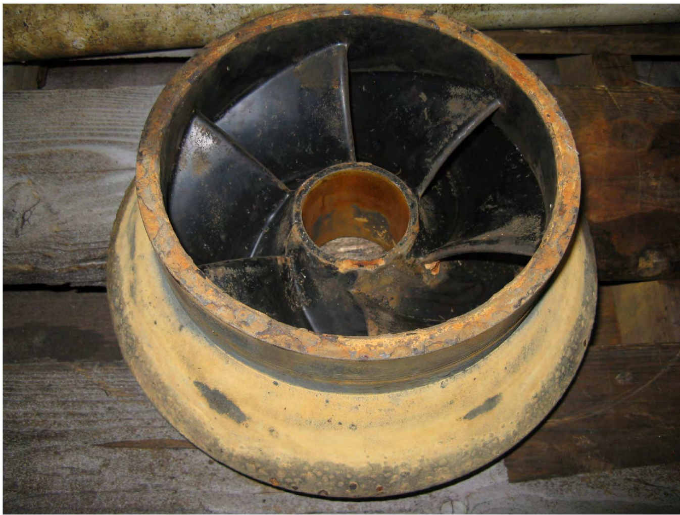
Picture #16 Back side of Impeller with herisite lining. The lining is acceptable for reuse.
