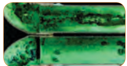
Pitting in 6-year-old cold water pipe caused by excess flux at solder joint.
