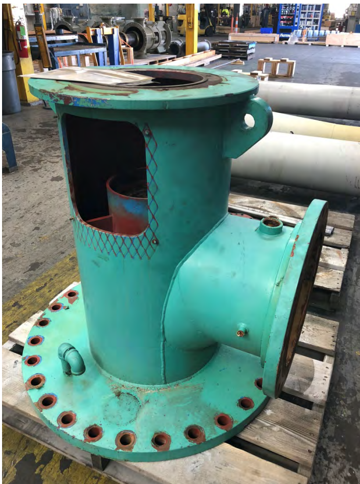
Picture #3 – The discharge head was inspected when removed. The head will be reused. Parts to be blast and recoated for protection.
