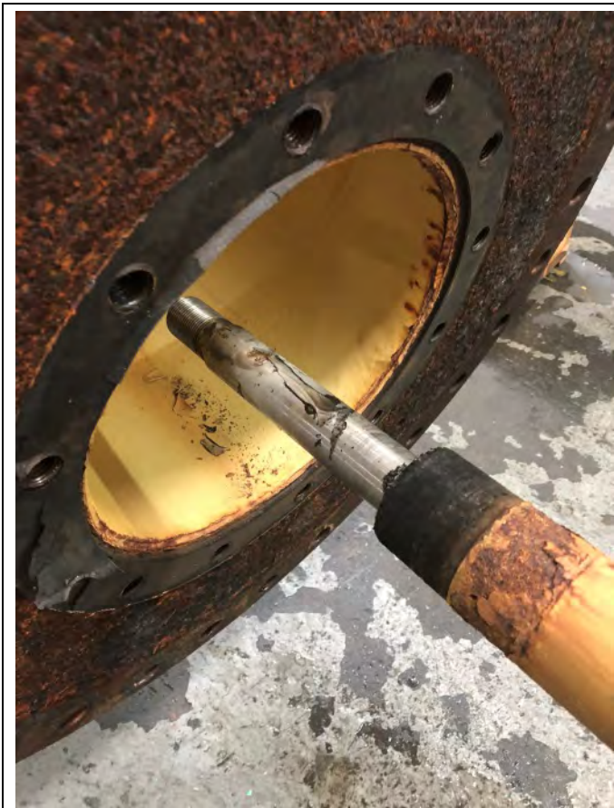
Picture #13 – Threaded connection of enclosing tube and the enclosing tube itself is reusable
