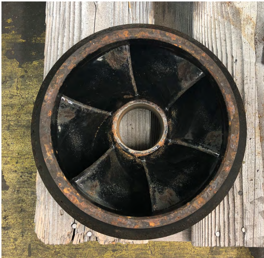
Picture #15 – The lining is in good condition. Floway recommendation will be to reuse with reconditioning of; steam cleaning and wire brushing. The external surfaces are to be blasted and recoated with the rest of the pump.
