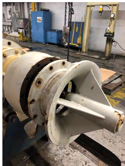
Picture #11 – Second picture of bell in relatively good condition given the pumps age. Nothing other than wear detected.
