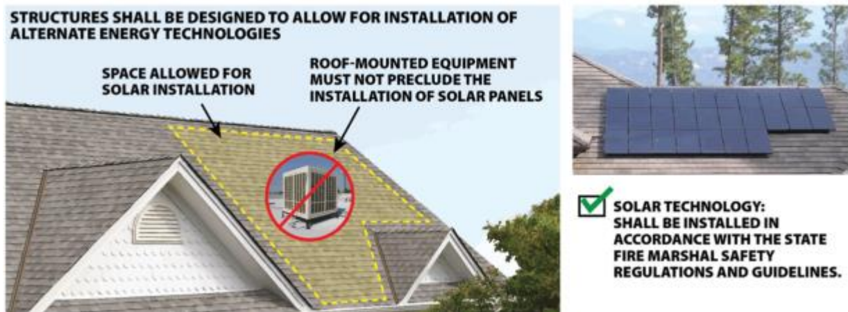
Figure 1-1: Application of Roof-Mounted Equipment
