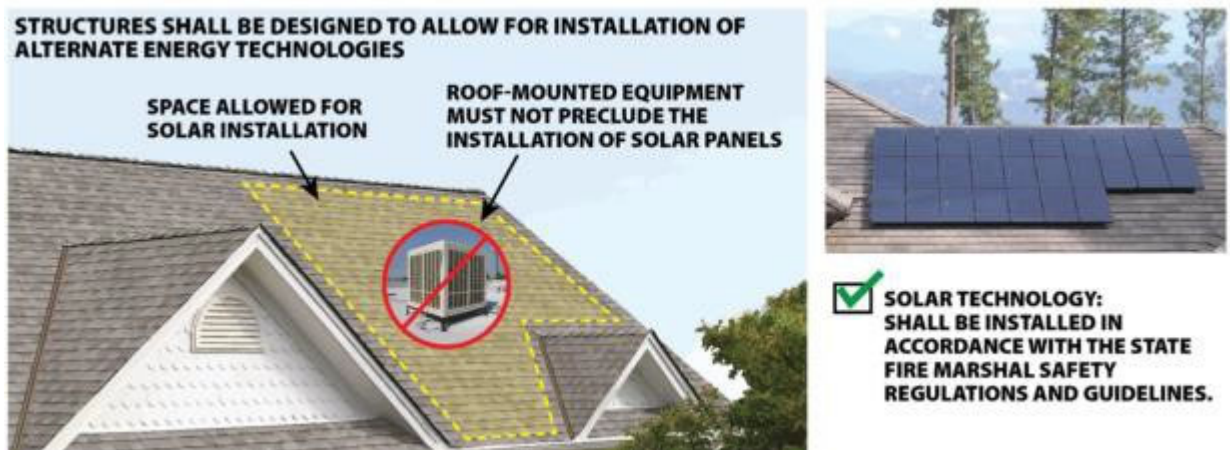
Figure 1-1: Application of Roof-Mounted Equipment
