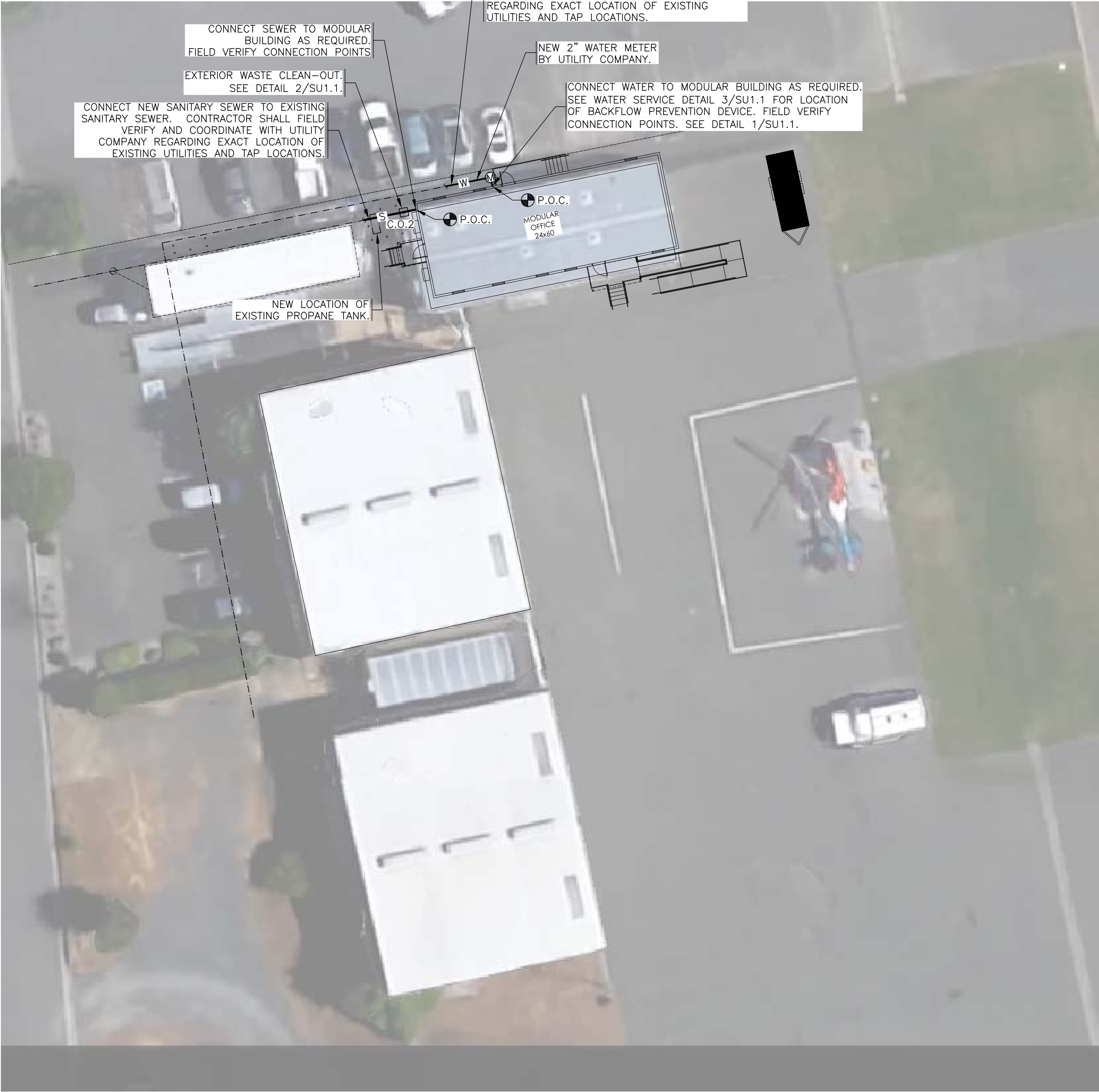
1 SITE PLUMBING PLAN SCALE: 1"=20'
