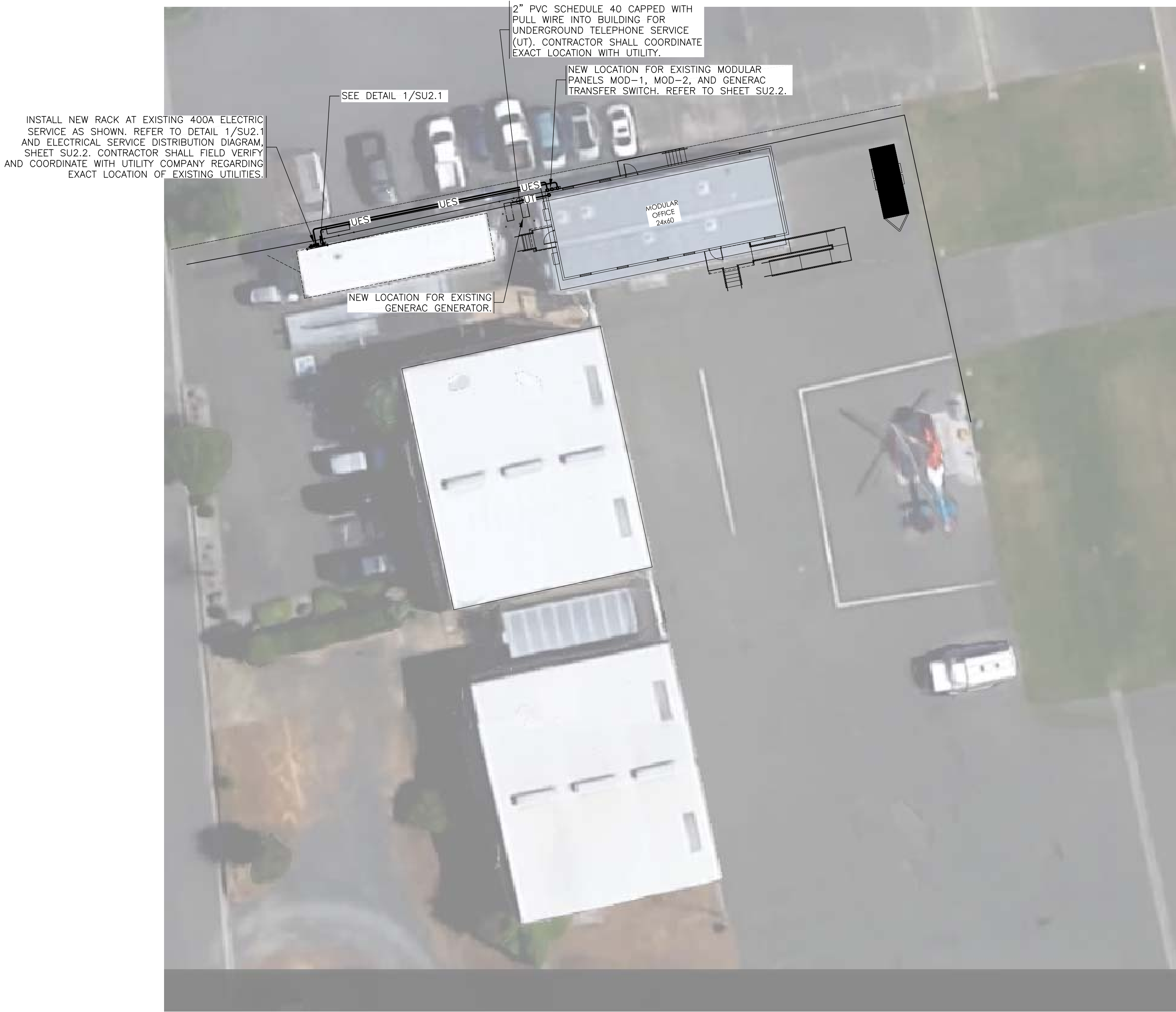
1 SITE ELECTRICAL PLAN SCALE: 1"=20'
