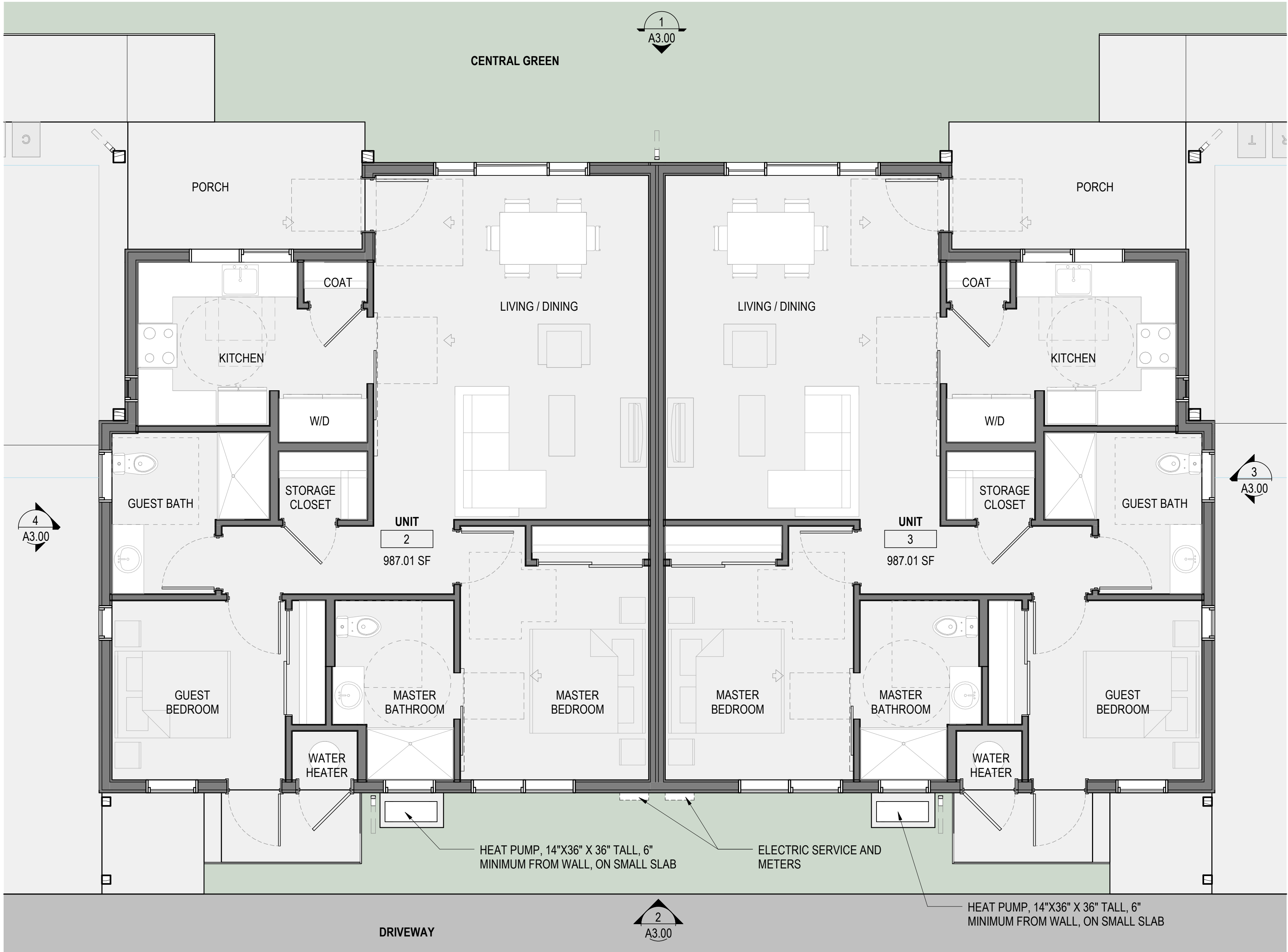
ENLARGED FLOOR PLAN_DUPLEX BLDG (SOUTH) 1 1/4" = 1'-0"
