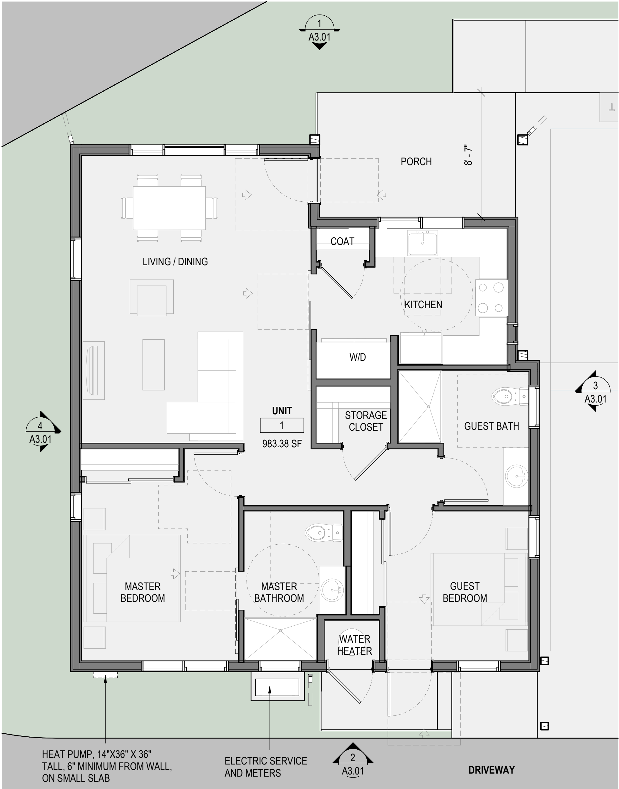
ENLARGED FLOOR PLAN_SINGLE BLDG 1 1/4" = 1'-0"
